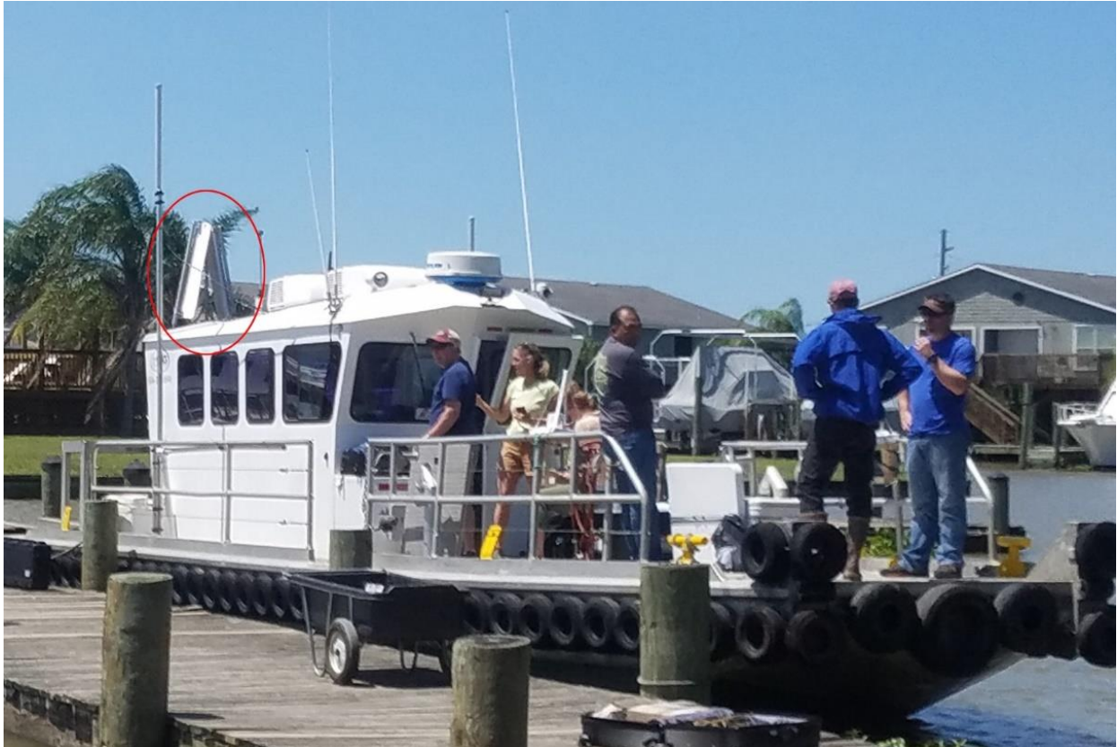
OI/MSRC communication system antenna installed on the 44-foot "Miss D" sampling vessel. Oil location, extent and thickness imagery/information were sent down from the aircraft within 10-15 minutes of data acquisition to the crew sampling the oil on the ocean's surface below.
