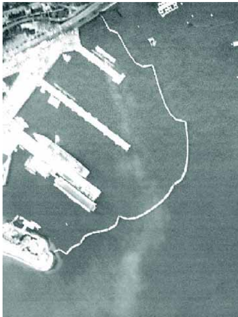
Fuel spill from a dock in San Diego Bay revealed by UV fluorescence.
