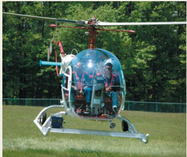
Our DMSC sensor mounted on the chopper skids taking off to image oil in the Ohmsett tank.
